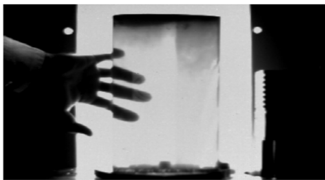
Fig. 1: SWIR InGaAs picture of a Si brick – note that the ingot is completely transparent for SWIR radiation.
